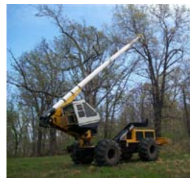
The Jarraff All-Terrain Tree Trimmer keeps Carroll Electric’s crew members safely on the ground while the trimmer’s fiber glass boom reaches cutting heights up to 75 feet.
